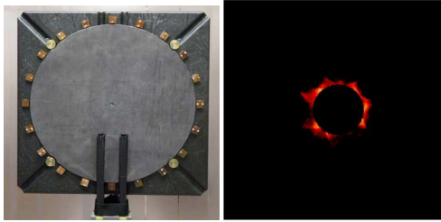
Fig. 1. Left: The second prototype built and tested in the small Larix Facility of the Ferrara University. Right: Focal spot of the second prototype compared with the expected PSF (black spot).
